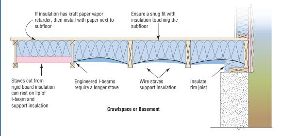
A stave is a mechanical method of supporting insulation from the bottom-up. Placing extra wire staves may be required to ensure adequate contact of the insulation with the subfloor even if it results in more compression of the insulation. Whether the insulation is oriented parallel or perpendicular to the rim joist, make sure the rim joist has full height coverage. Consider removable insulation to allow for pest and termite inspection.
